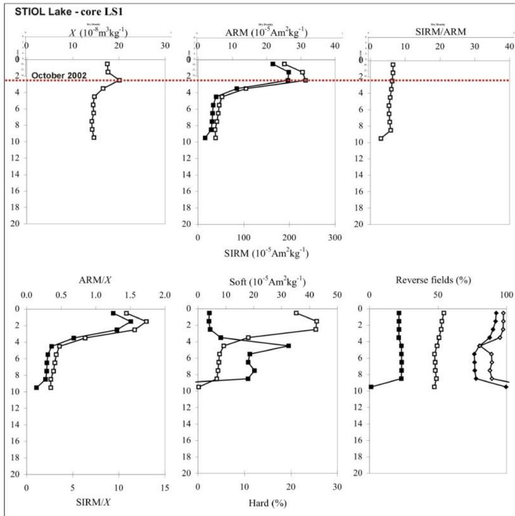
Fig. 1.4.3. Mineral magnetic properties of a short sediment core from post dam Lake Stiol (core LS1) (Key: SIRM, SIRM/ $X$  and Hard shown as solid symbols. Reverse field measurements at -20mT (closed squares), -40mT (open squares), -100mT (closed diamonds) and -300mT (open diamonds).
