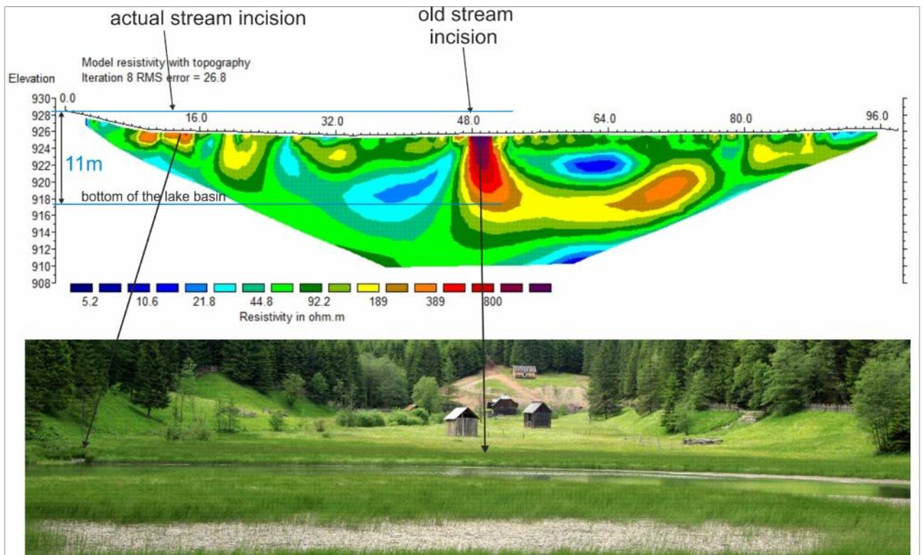
Fig. 1.3.11. Electrical resistivity tomography (ERT) survey on a landslide-dammed lake (Iezer-Feredeu lake, Obcina Ferdeu Mts).
