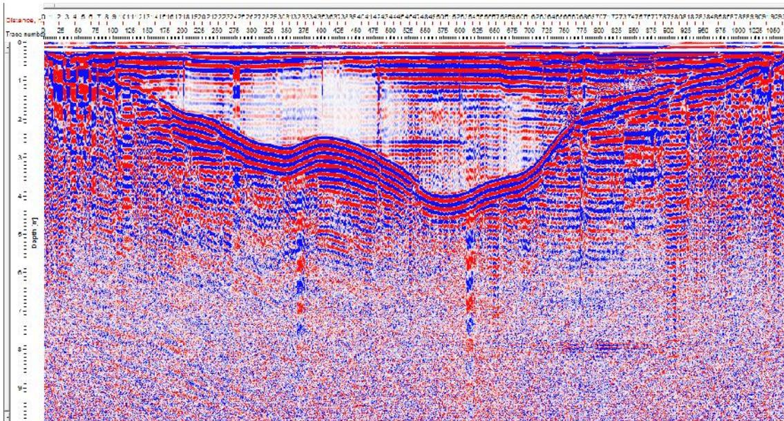
Fig. 1.3.7. A ground-penetrating radargram collected on Iezer lake (Lesenciuc et al., 2010).
