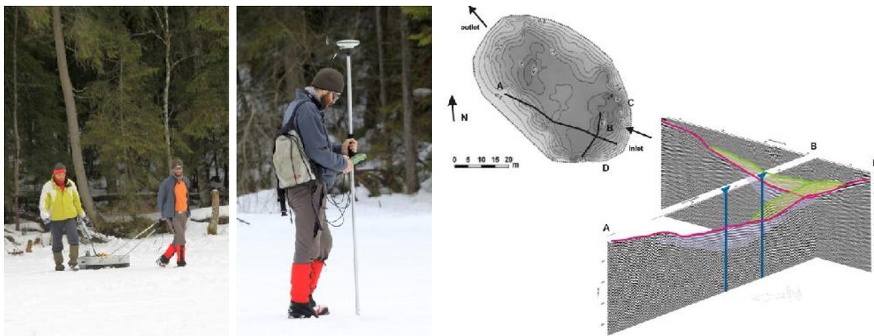
Fig. 1.3.5. Left: GPR survey on Bolătău lake (March 2014). Right: routes used in order to intersect the core points and correlate the cores.
