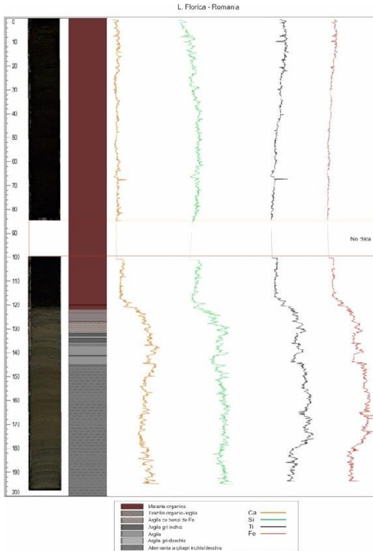
Fig. 1.3.17. XRF profile (Ca, Si, Ti, Fe) of sediments from Florica lake.
