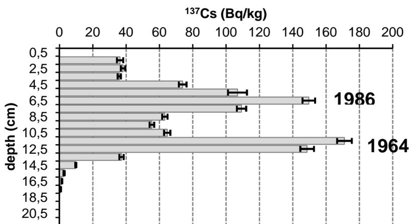
**Fig. 1.3.24.** Radiocaesium specific activities along the 20 cm topmost section of the Bolătău sediment sequence. Whiskers indicate the estimated analytical error. The distinct concentration peaks supposed to be coincident with 1986 (Chernobyl accident) and 1964 (north hemispheric fallout maximum) are indicated.
