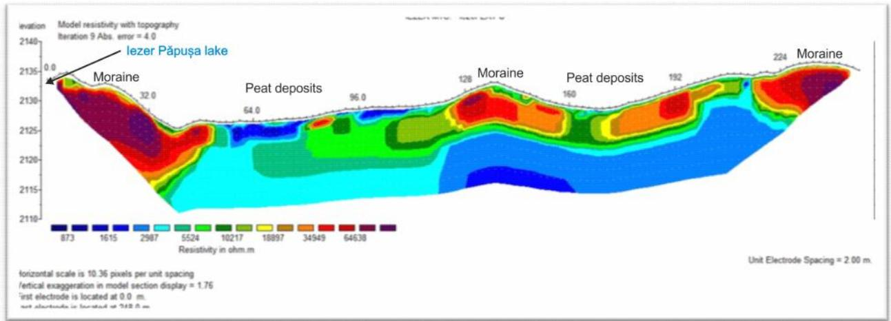
Fig. 1.3.10. Electrical resistivity tomography (ERT) survey on glacial cirque floor (Iezer cirque and lake, Iezer-Păpușa Mts).
