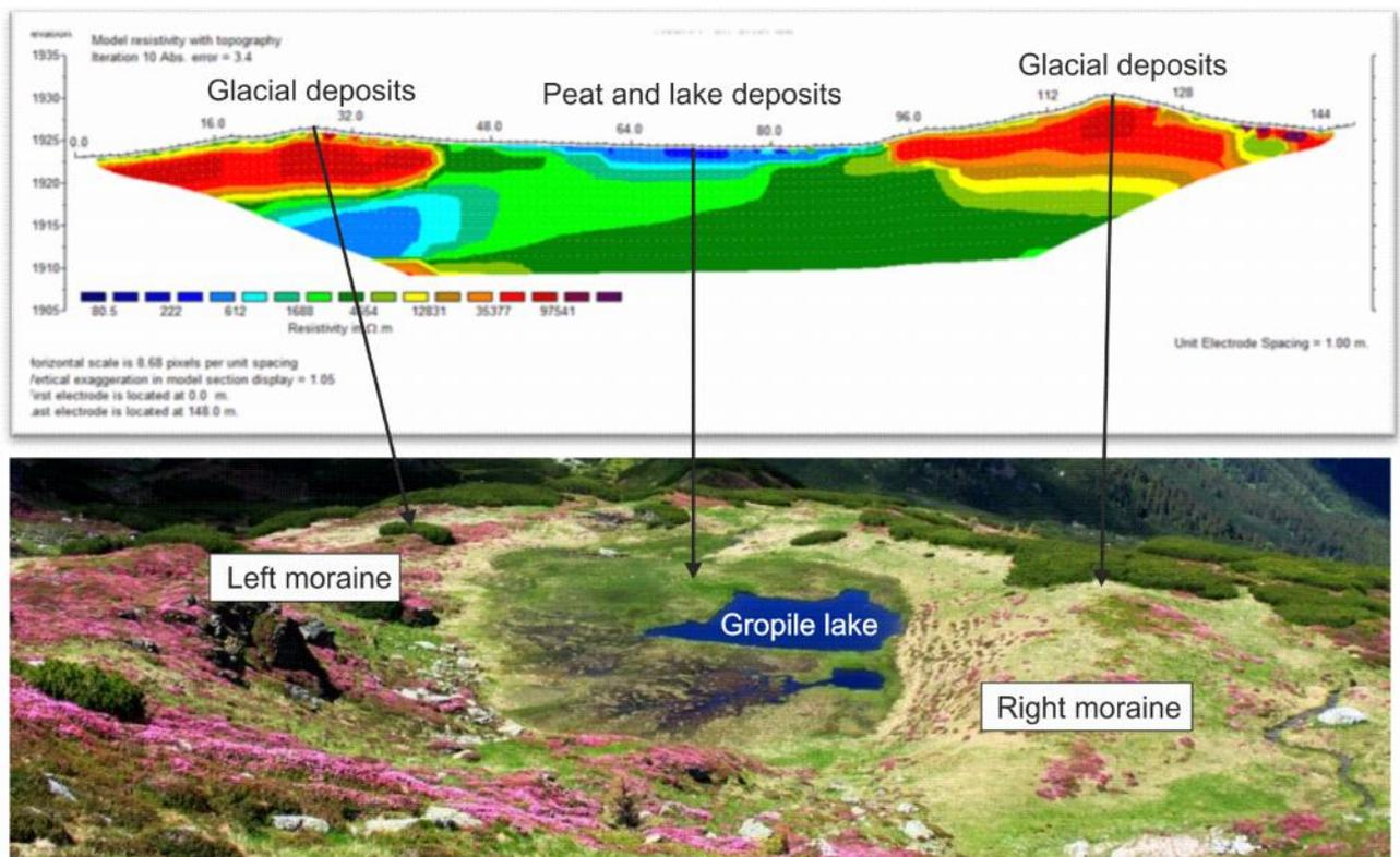
Fig. 1.3.9. Electrical resistivity tomography (ERT) survey on glacial lake and deposits (lake Gropile, Rodna Mts).
