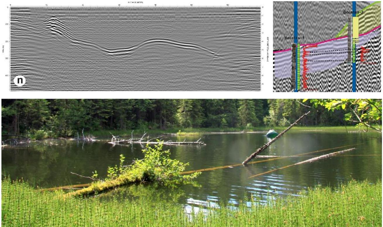
Fig. 1.3.6. Left: A ground-penetrating radargram collected on Bolătău lake. Lineations indicate the presence and extent of sediments layers. Right: Position of the cores and how they integrated into GPR profile based on marked layers (cores correlation as well). Below: Bolătău lake.
