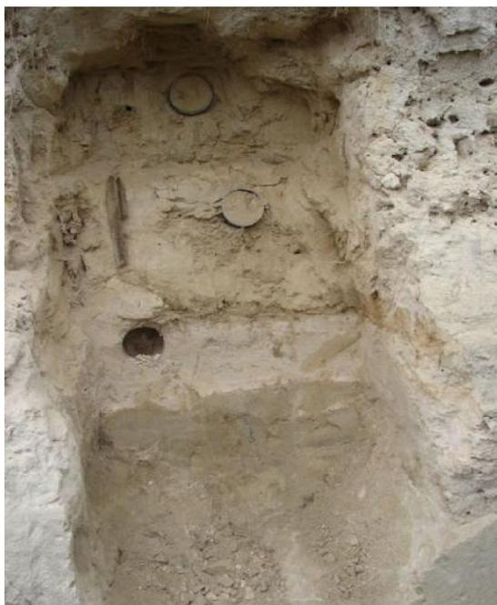
Figure 1.3.25. OSL sampling using plastic tubes.
