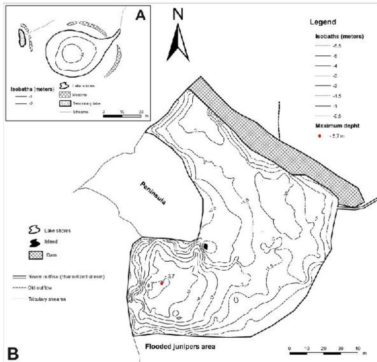
Fig. 1.3.4. Comparison of bathymetric surveys of Lake Ştiol. A. pre dam (according to Pişota, 1968); B. post dam.
