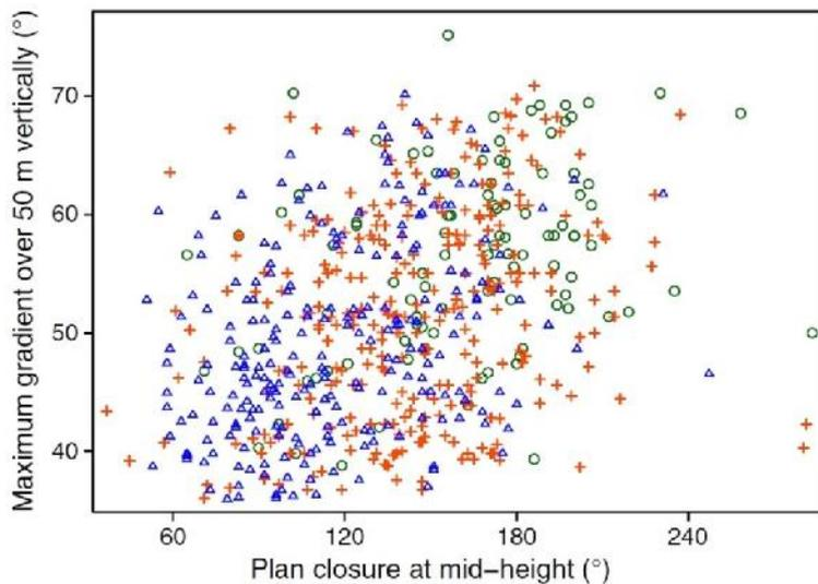
Fig. 2.4.4. The weak relations between plan closure, maximum and minimum gradient. Triangles: minimum gradient  $\geq 10^\circ$ ; crosses: below  $10^\circ$  but  $\geq 0^\circ$ ; circles:  $0^\circ$ .
